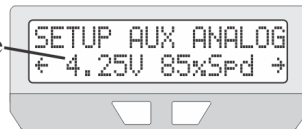
Analog Potentiometer Set for Adjusting Max Speed Limit.
