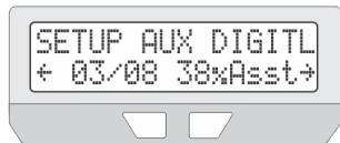
Digi Aux Set for 8 Levels of PAS Assist. Currently on Level 3 (38% of Max)
