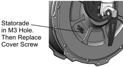
Statorade is injected into the motor from a small M3 screw hole located on the right side plate. Add Statorade with a syringe tip with the hole on the bottom so that the fluid flows directly downwards and into the rotor magnets and avoids flowing over the motor bearings and torque sensor. Remember to put the screw back in to seal the hole.
