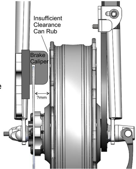
Figure 13: Illustration of Caliper Clearance.
